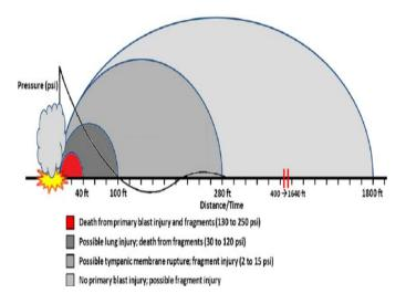
In general, if we want to put a general model for basic safe distances, Figure 5 describes the effective firing power, kill radius and injury radius. Generally to maintain a safe distance regarding most mines, the base station controller must be around 300 meters far from the mine field.
